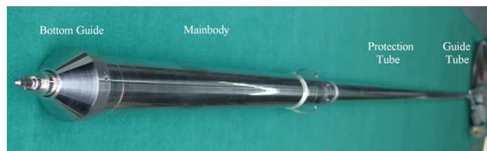
Fig. 1. Instrumented capsule for the material irradiation tests.
